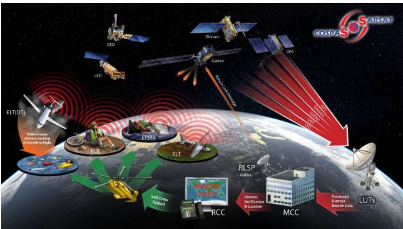
Figure 2. COSPAS-SARSAT System. Source www.COSPAS-SARSAT.int
